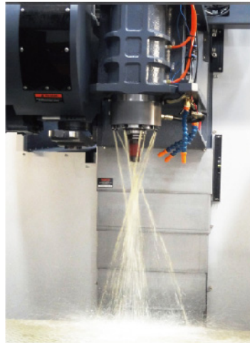
Spindle Annular Coolant Jet with 8 Nozzles
